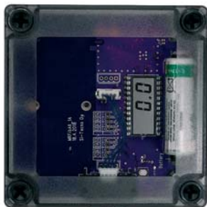
Wireless sensor for measuring indoor atmospheric pressure.
